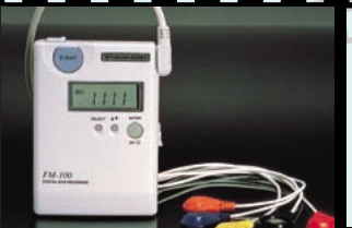
Holter ECG Recorder FM-100 Produced from 1995, a lightweight and super-compact body
