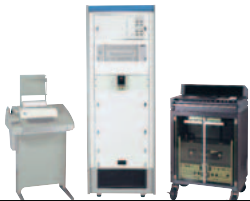
Computerized Automatic ECG Analysis System ECP-100 Produced from 1977, ECG and Mini-computer combined Automatic ECG analysis system
